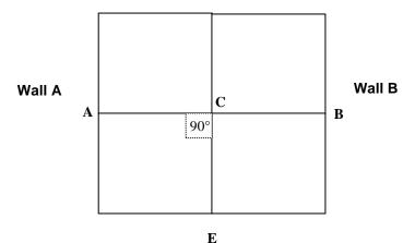
6.4 Starting at center point C, measure out the length and width to the walls to make sure you will have at least a half of a tile at the border. Adjust lines A-B and D-E if necessary.
