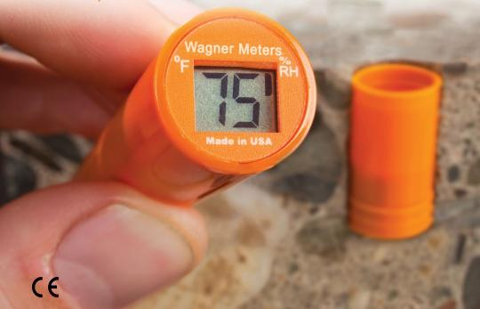
The Rapid RH® moisture testing system should be used on any project where moisture-sensitive floor coverings or coatings are to be applied over concrete slabs. Owners, general contractors, flooring contractors/installers and testing companies need to be sure the tests they perform are accurate, repeatable and available to all who need to know the current moisture condition of concrete slabs.
