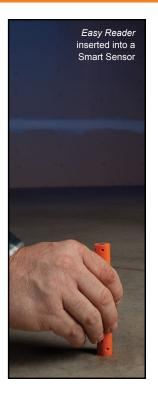
After the initial equilibration has been reached per ASTM F2170 requirements, subsequent readings can be taken instantly (see ASTM F2170 Best Practices section at the end of this manual). If future testing is needed, replace the protective cap by snapping it back into the Smart Sensor.
