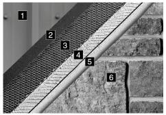
[1] Untreated/unpainted masonry concrete, [1] Rigid foam insulation, [2] SM-BT, [3] [1] Metal building, [2] SM-BT, [3] Galvanized metal lath, [4] Mortar/scratch coat, [5] Mortar setting bed, [6] NTSV
