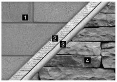
[2] Mortar/scratch coat, [3] Mortar setting Galvanized metal lath, [4] Mortar/scratch bed, [4] NTSV
