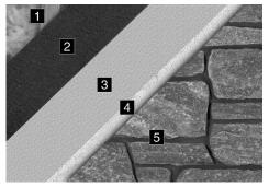
[1] Wood or steel studs, [2] SM-BT, [3] Cement board, [4] Mortar setting bed\*, [5] NTSV
